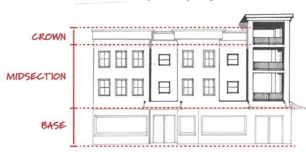
FIGURE 9.2 TRIPARTITE (3-PART) FAÇADE DESIGN
